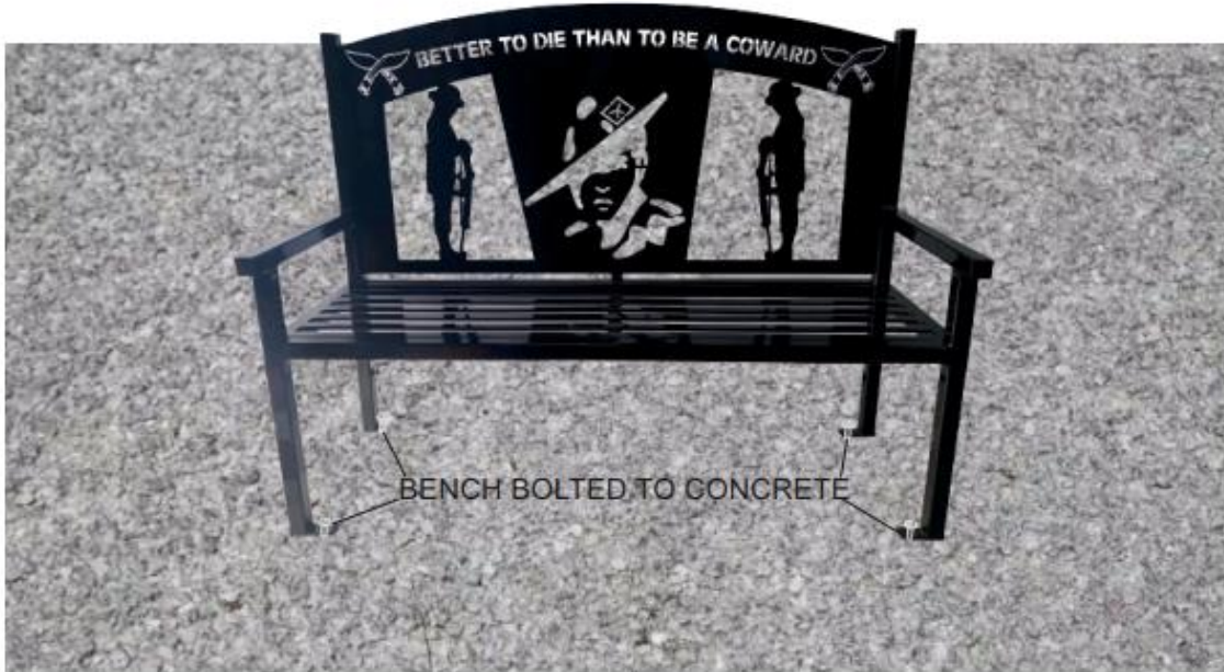
Concrete Pad and Bench Securing
