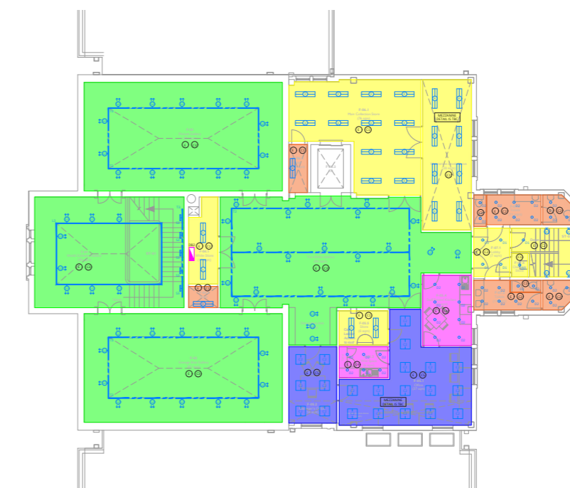
First Floor Lighting Layout
