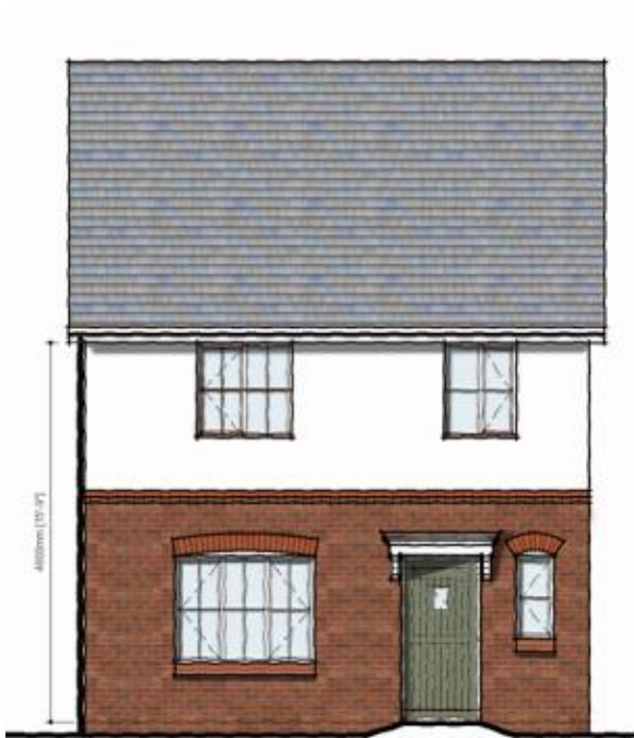
Front Elevation 6.1 (Brick/Render) Scale 1:100
