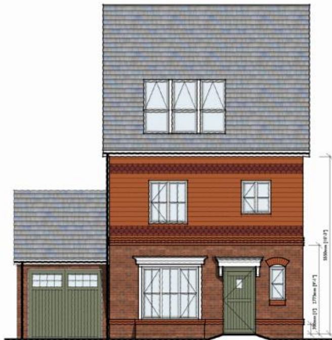
Front Elevation 6.2 (Brick/Tiles)
