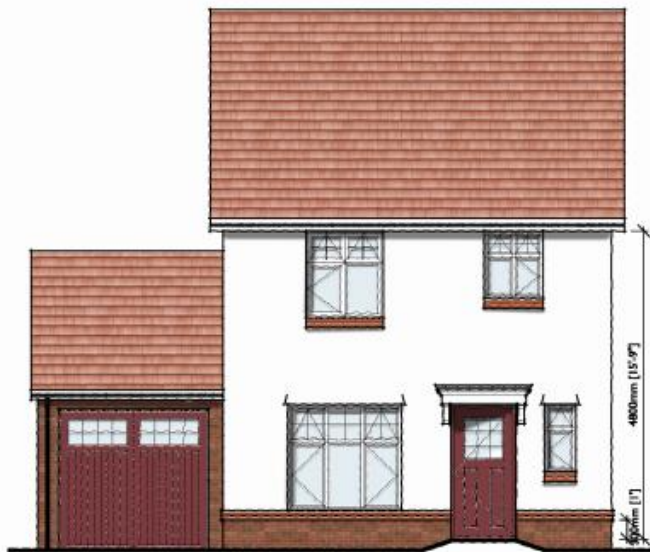
Front Elevation 6.1 (Brick/Render) Scale 1:100
