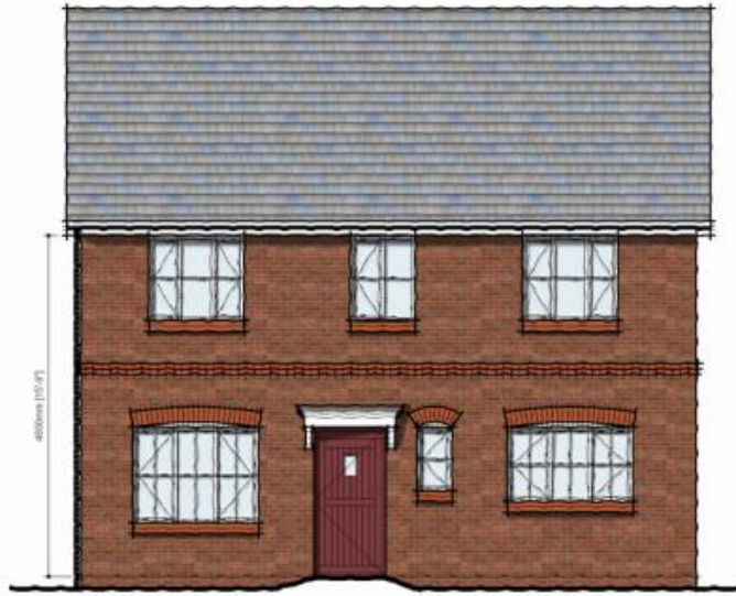
Front Elevation 6.0 (Brick)
