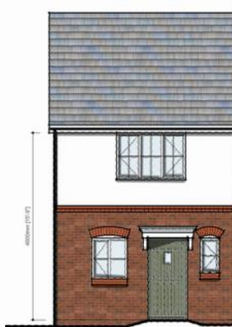
Front Elevation 6.1 (Brick/Render) Scale 1:100
