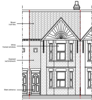
01 PRE-EXISTING FRONT ELEVATION 1:100(A3)
