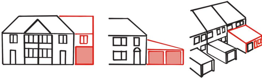
Figure 26: Extensions unsympathetic to the original roof form of the house
